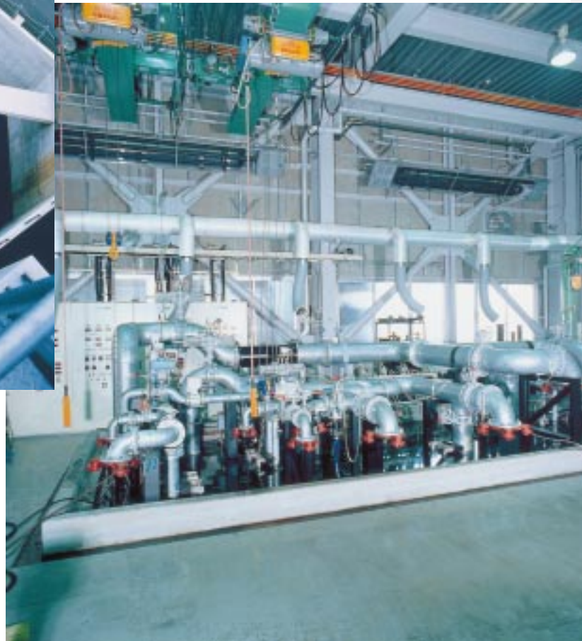
Performance testing apparatus for medium-sized pumps
