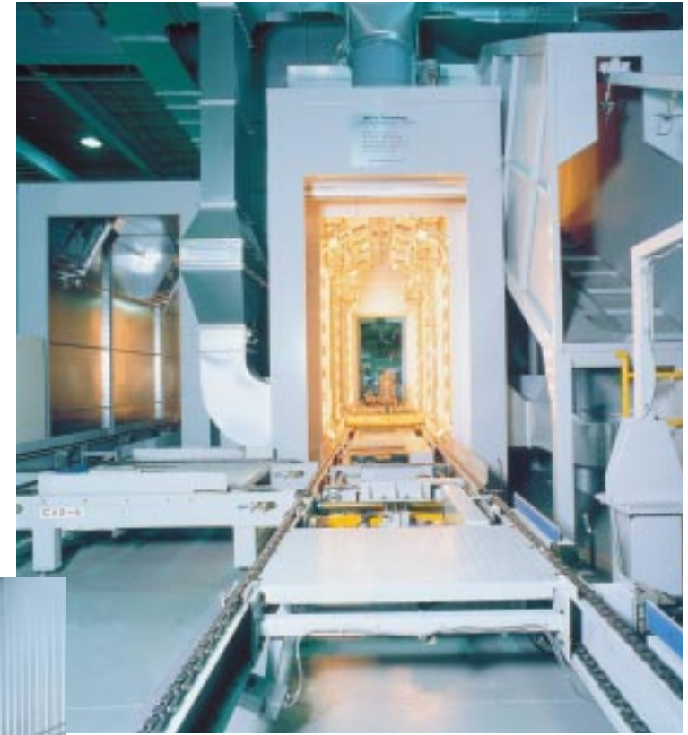
Painting line for special pumps
